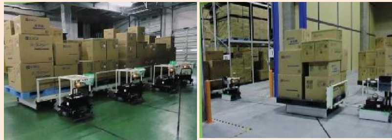
Unmanned transfer along the designated route on the same floor of the warehouse
