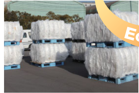
Once sorted, transparent containers are pressed into bundles with a newly installed compressor. This allows many containers to be transported at once.
