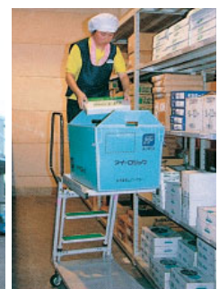
A newly developed picking cart for high shelving
