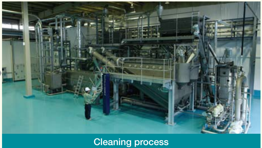
Impurities are removed by a final separation of caps and labels and by alkaline washing.
