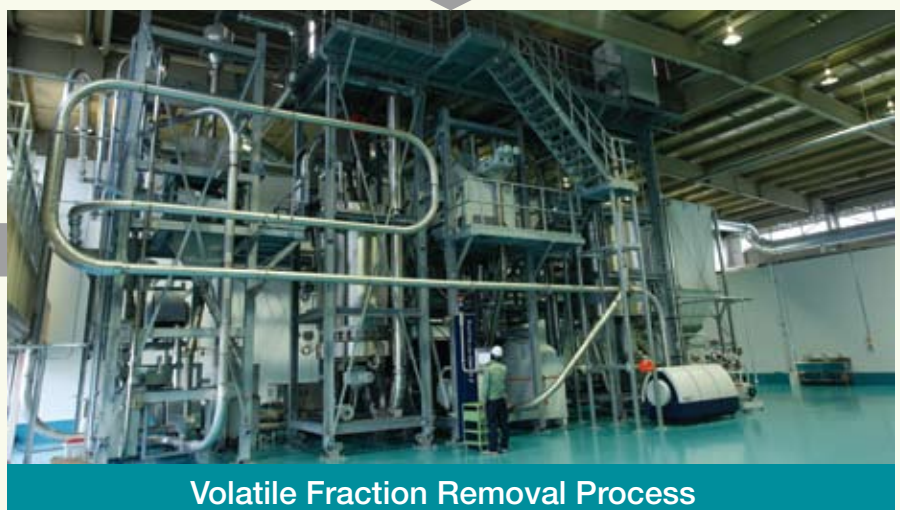
Volatile fractions are removed while the material passes slowly through a high-temperature vacuum reaction furnace.
