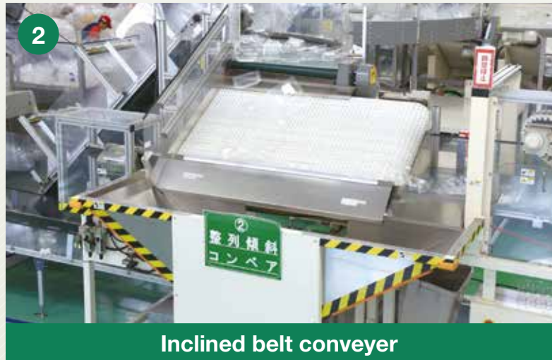
Flow volume is controlled using an incline.
