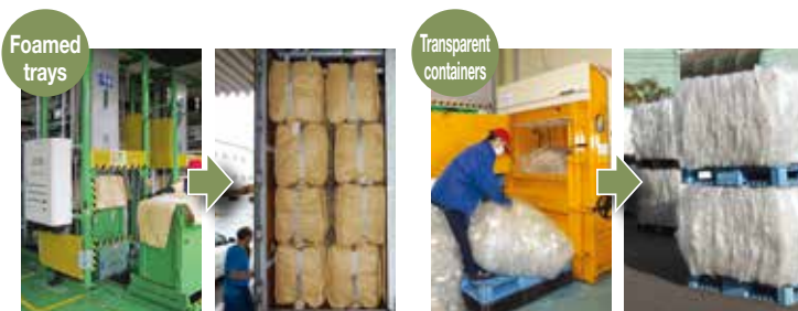
After the sorting process, trays and containers are compressed to substantially reduce their volume
