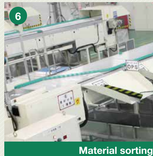
The sorter sorts the containers by material.
