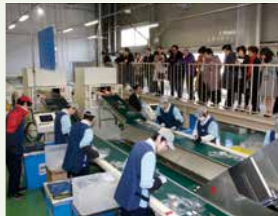
Process of sorting used transparent containers, in which workers with disabilities are deployed
