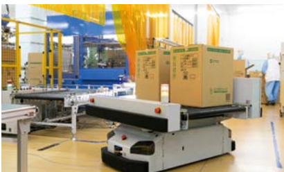
(3) Cases of products are loaded onto an automatic guided vehicle (AGV) and carried a short distance to the conveyor.
