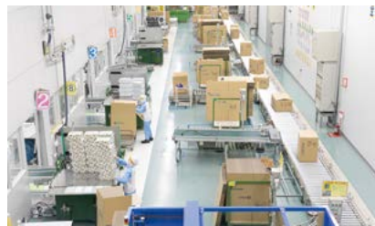
(4) Cases of products are successively loaded onto the conveyor and collected at a depot.
