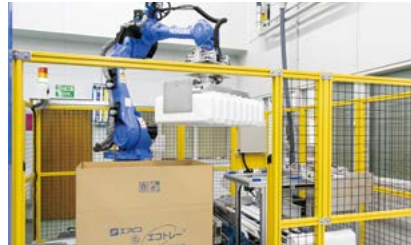
(2) Packed products are lifted by a robot arm for containers. A predetermined number of products are placed into a cardboard case.
