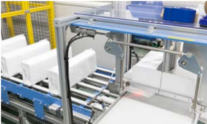
(1) After cutting, products are packed into plastic bags by the automatic packaging machine. Then, they are transported by conveyor.
